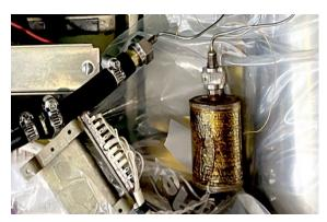
Upon turning on the gas for a trial run at room temperature, my initial impression was unsettling. Most literature indicates that the gas-absorption process is noticeably exothermic, requiring cooling during the refilling process to keep the reaction going. But the canister didn't seem to warm up . A DMM connected to the thermistor at pins 3 and 4 of the associated connector did not indicate any internal temperature rise at all.
