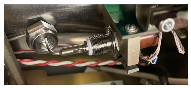
After unscrewing the line at the pressure sensor, I immediately covered its end-face aperture with a piece of Kapton tape. I then proceeded to disassemble the bracket and clamp holding the canister in place so that I could measure the threads on the pressure sensor back at the workbench. So far, so good... but at some point the tape came off.
