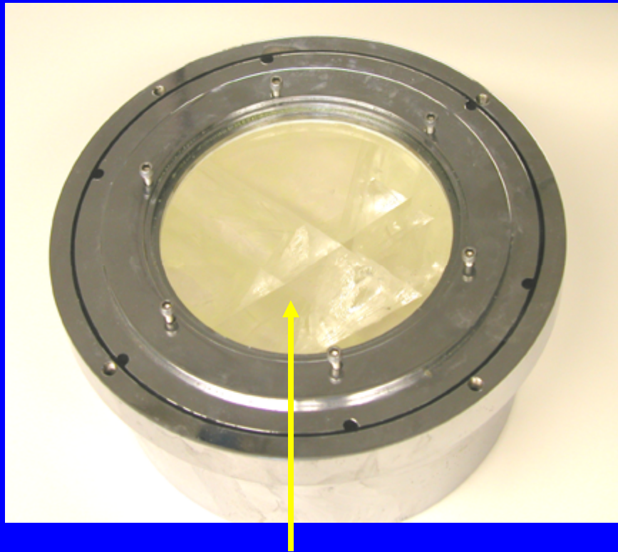
Cracked NaI Crystal
