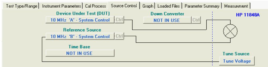
For Test Type Phase Noise Without a Phase Locked Loop, the Source Control Tab looks like this:
