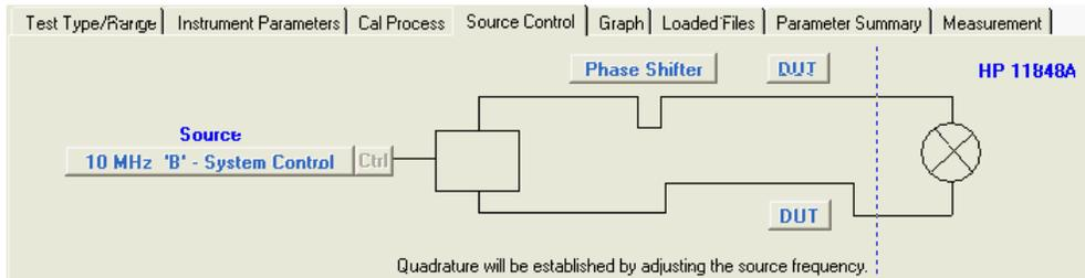
For Test Type Phase Noise Using an FM Discriminator, the Source Control Tab looks like this:
