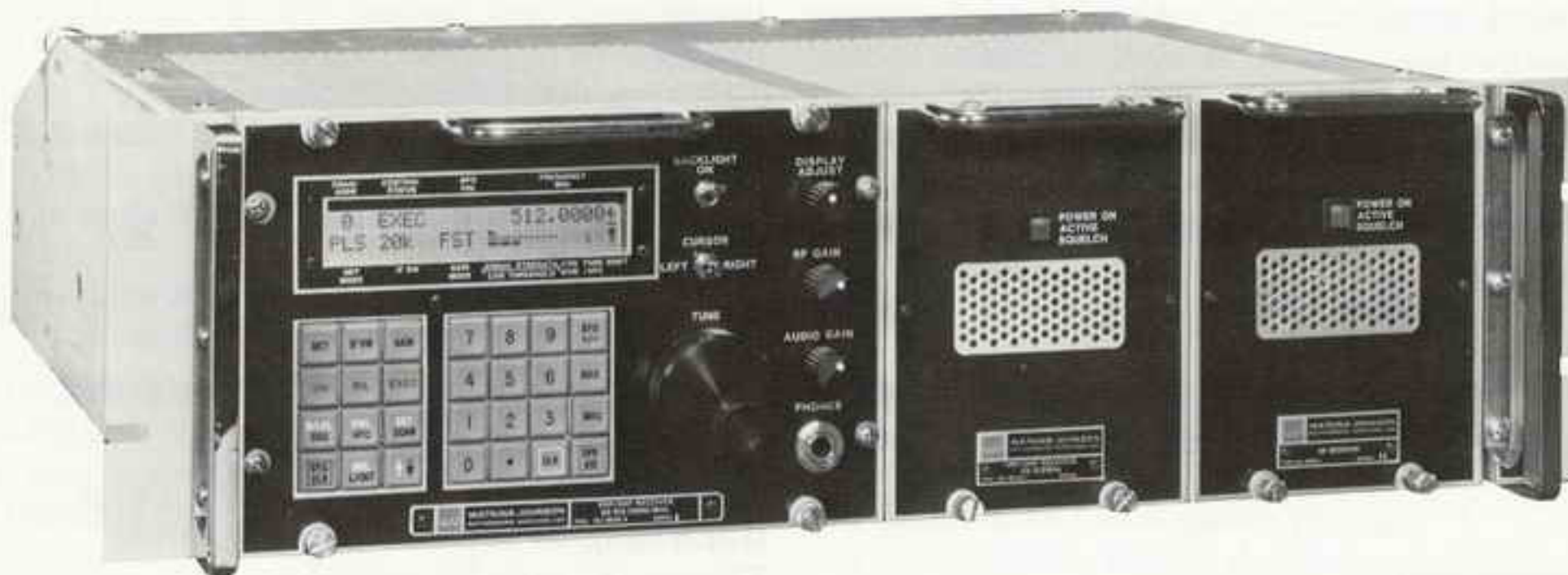
Figure 2 WJ-8628A-4 Configured With a WJ-8628A-1 and WJ-8626A-1 In a 5 kHz to 2000 MHz Master/Slave Subsystem
