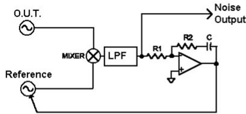
$$\omega = \sqrt{\frac{k_{\phi} k_v}{R_1 C}}$$
