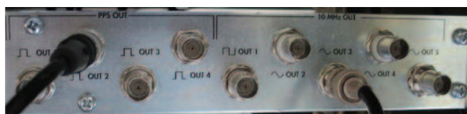
Figure 7. Back panel of a GPSDO with multiple output signals.
