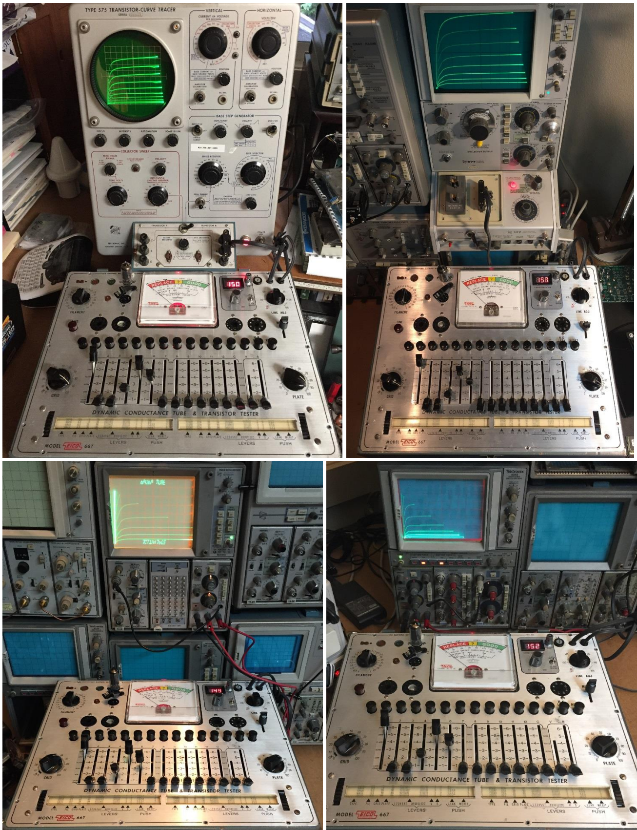
Figure 11 Clockwise from upper left: displaying the 6AU6A characteristic curves on a 575, a 577, a 5CT1N plugin, and a 7CT1N plugin. The 6mA current limit and fixed load resistors of the 7CT1N / 5CT1N mean the plate voltage can only swing part way across the CRT for the 0V to -2V grid steps.
