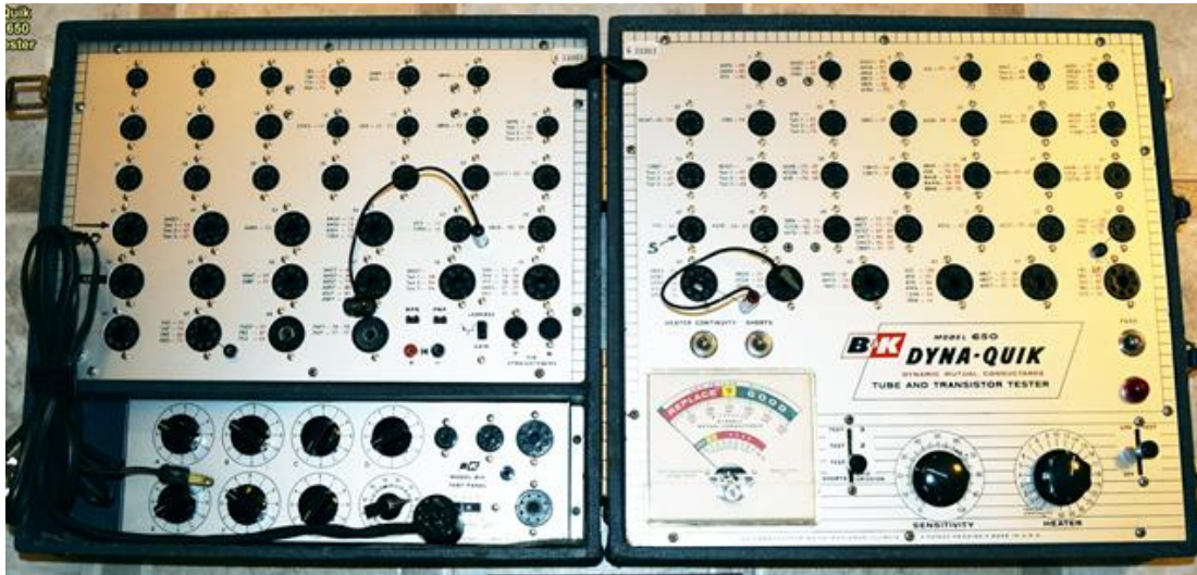
Figure 3 B&K DynaQuik Dynamic Mutual Conductance Tube and Transistor Tester. Note the large number of sockets which minimizes test setup time and setup errors.
