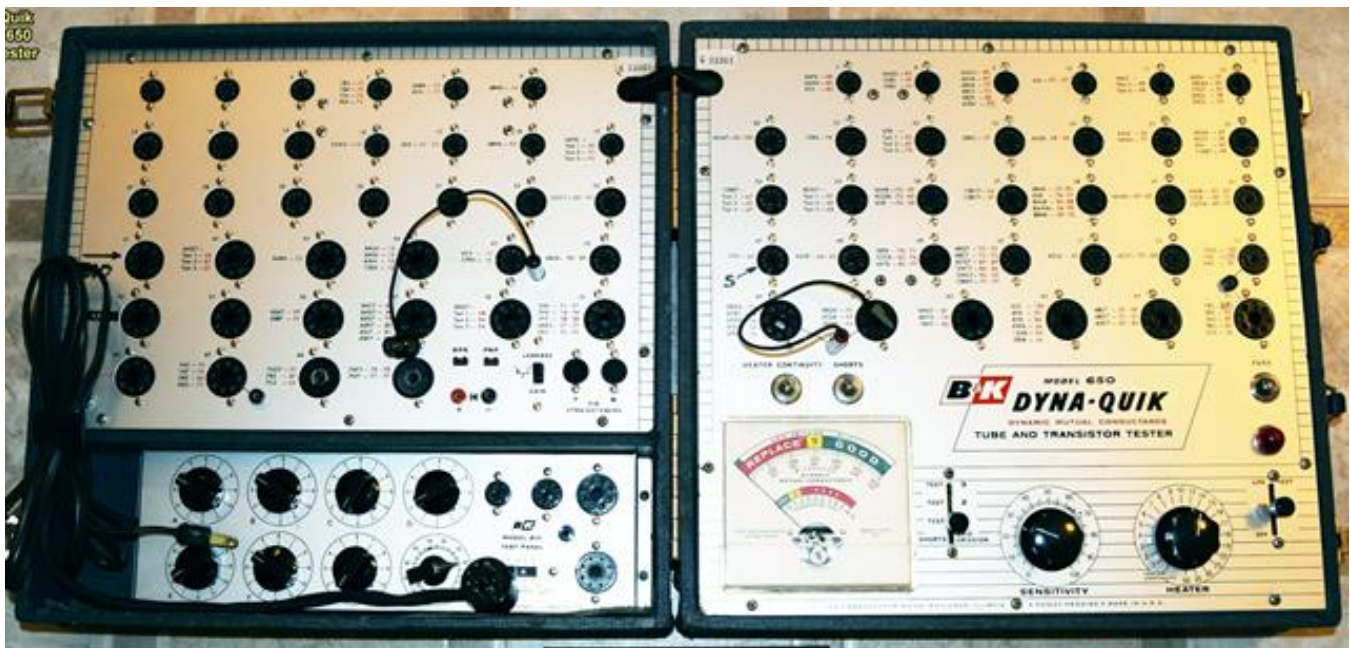
Figure 5 B&K DynaQuik Dynamic Mutual Conductance Tube and Transistor Tester. Note the large number of sockets which minimizes test setup time and setup errors.
