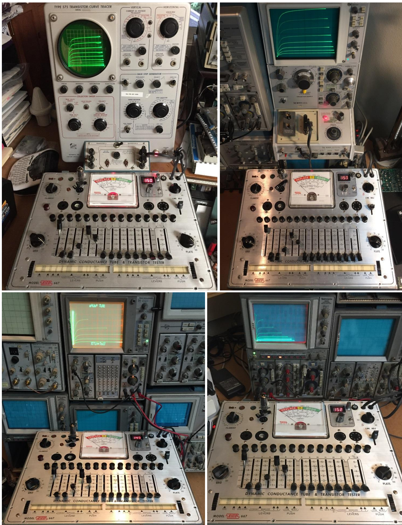
Figure 13 Clockwise from upper left: displaying the 6AU6A characteristic curves on a 575, a 577, a 5CT1N plugin, and a 7CT1N plugin. The 6mA current limit and fixed load resistors of the 7CT1N / 5CT1N mean the plate voltage can only swing part way across the CRT for the 0V to -2V grid steps.
