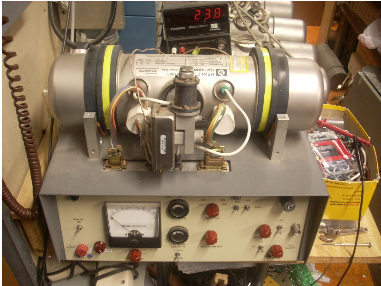
"Mini" tube in Cesium tube test set, note black plastic fittings
